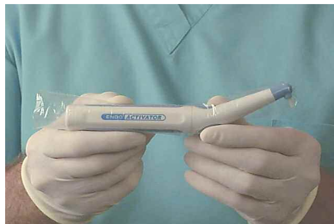
Figure 11. Custom EndoActivator barrier sleeves are designed to slide over the entire handpiece, including the driver.
